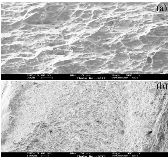
**Figure 3 SEM fractographs (a) 35 % RH air (b) synthetic seawater C276 in 30 % cold rolled condition. Strain rate  $10^{-6} (s^{-1})$**
