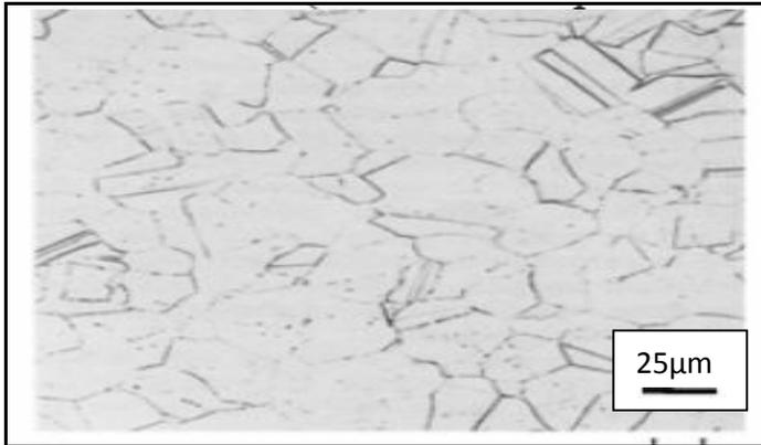
**Figure 1 Optical microstructure of Alloy C276 after cold rolling. Etchant: Glyceregria 15cc HCl + 10cc Glycerol + 5cc HNO<sub>3</sub>.**
